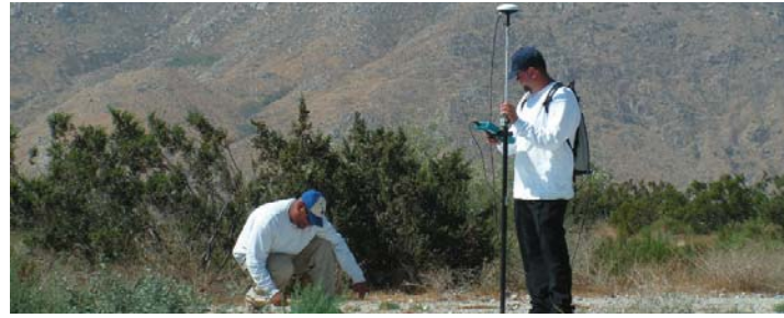
Using StarFire, the SPEC team pinpointed and set the location of about 300 aerial survey control panels.
